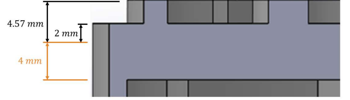
Fig. 9. New minimum and maximum thicknesses of the soundboard with braces added. View of body taken below the bridge where thickness was increased entirely across the body.
