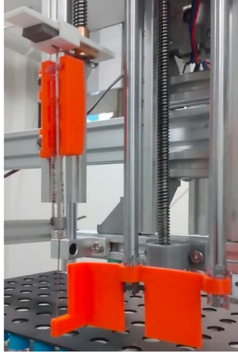
FIGURE 9.4.1: EXAMPLE OF NEEDLE CLAMP AND NEEDLE GUIDE IMPROVEMENTS
